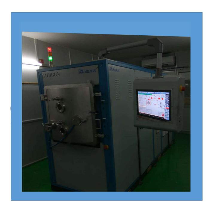
The **Compact Coater** is an Industrial Coating system based on **Magnetron Sputtering Technology** designed for Sputter deposition of films of low thickness on cutting edges of Double Edge Shaving Blades. Basic coatings offered are Cr (Chromium) followed by CrN (Chromium Nitride). Platinum sputter coating or DLC (Diamond Like Carbon) coating facility can be provided on request.
