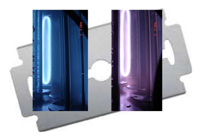
**Substrate Table:** Table is dedicatedly designed to have 30 stations. Each station holds 3000 numbers of 0.1 mm thick double edge razor blades. The blades can be easily stacked together on the rigid stainless steel support thus exposing sharp edges of the razor blades to be coated to vapour sources. The total loading capacity therefore is 90000 for double edge and 120000 for single edge blades.
