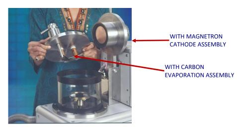
The assembly can be directly adapted to the MILMAN 'SEMCOATER'.
